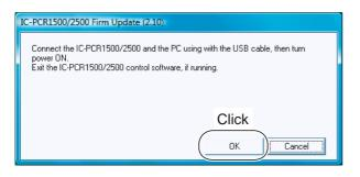
(5) Connect the Main unit and the PC using the USB cable, and turn the Main unit ON.
